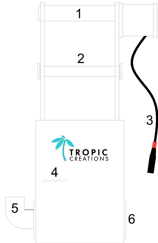
Attention! The non-woven fabric should be attached to the roller with the motor with a sticker which is attached to the new roller marked Roller clean 100, the non-woven fabric should be placed on the roller with the motor, and after turning the motor one full turn, the fleece will tighten on the motor. The motor itself can be mounted on the left or right side (3)
